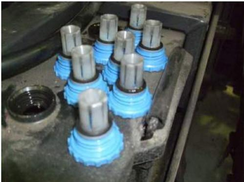
Pictured above are battery caps from one of our lead-acid batteries that have been in use for 2 years. As evident the caps are completely clean and free from sulfation, something that has kept the battery "like new" and yielding the rated power of 225Ah.
